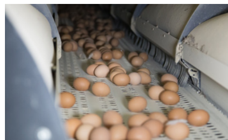
Extra-wide center located egg belt allows room for eggs to roll out, resulting in less cracks
